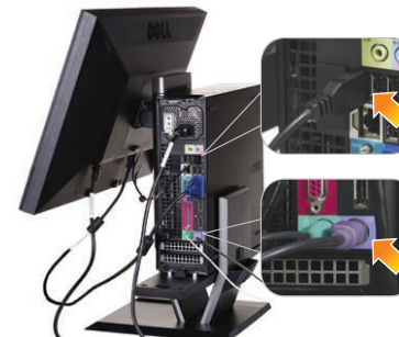
7 Connect the USB, keyboard and mouse cables to the computer as shown
